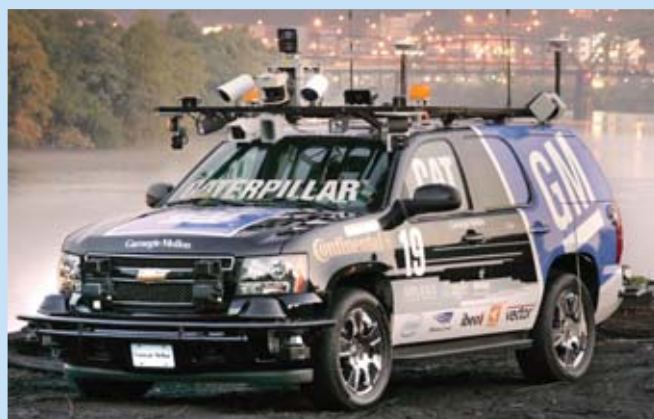
DARPA Urban Challenge 2007: Boss, the Tartan Racing robot, is built on a Chevrolet Tahoe chassis. It incorporates lidar, radar and visual sensors to safely navigate urban environments.
